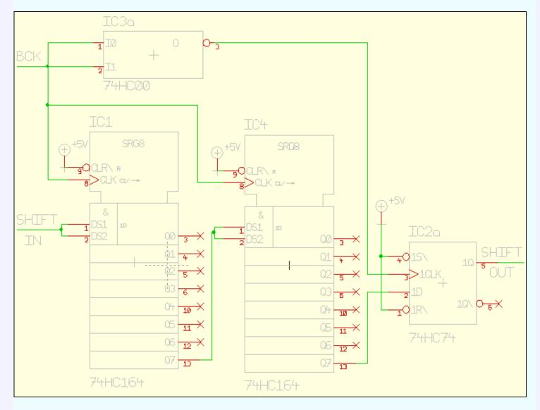
Q7 (IC1) puts out the signal present on "SHIFT IN" delayed by 7.5 BCK cycles.
