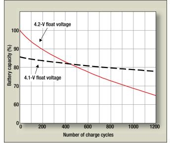
**Fig. 3.** The choice of a 4.1-V or 4.2-V float voltage impacts the battery capacity and the number of charge cycles.
