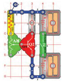
**OBJECTIVE:** To compare transistor circuits.
