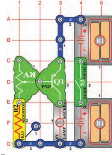
**OBJECTIVE:** To *demonstrate adjusting the* gain of a transistor circuit.
