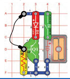
**OBJECTIVE:** To build a transistor light alarm.
