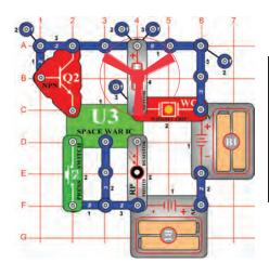
**OBJECTIVE:** To build a fan with sound that is activated by light.
