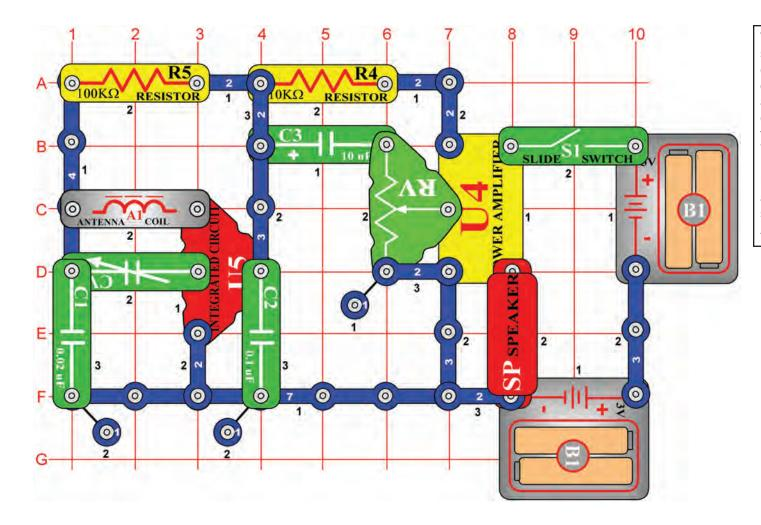
When you turn on the slide switch (S1), the integrated circuit (U5) should amplify and detect the AM radio waves all around you. The variable capacitor (CV) can be tuned to the desirable station. Varying the adjustable resistor (RV) will make the audio louder or softer. The power amplifier IC (U4) drives the speaker (SP) to complete the AM radio project.
