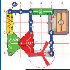
**OBJECTIVE:** To compare transistor circuits.
