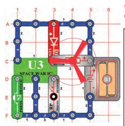
**OBJECTIVE:** To vary the speed of a fan activated by light.
