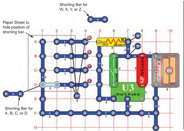
Build the circuit shown on the left. It uses two (2) 2-snap wires as shorting bars.
