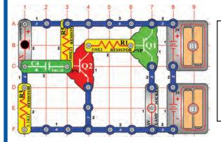
Install the parts. The lamp (L2) will be on. It will be off as long as you blow on the mic (X1). Speaking loud into the mic will change the brightness of the lamp.
