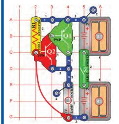
This light alarm circuit uses two transistors (Q1 & Q2) and both sets of batteries. Build the circuit with the jumper connected as shown, and turn it on. Nothing happens. Break the jumper connection and the lamp (L2) turns on. You could replace the jumper with a longer wire and run it across a doorway to signal an alarm when someone enters.
