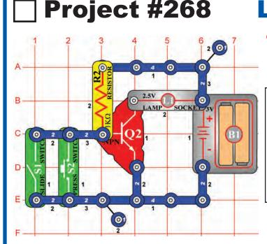
**Light NOR Gate** *OBJECTIVE: To build a NOR gate.*
