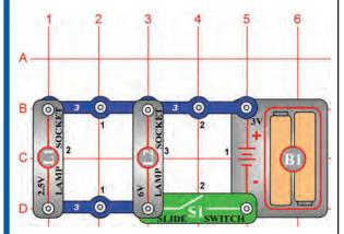
Turn on the slide switch (S1) and both lamps (L1 & L2) will light. If one of the bulbs is broken then the other will still be on, because the lamps are in parallel. An example of this is most of the lights in your house; if a bulb is broken on one lamp then the other lamps are not affected.
