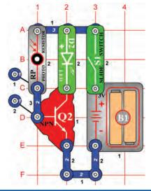
**OBJECTIVE:** To compare transistor circuits.
