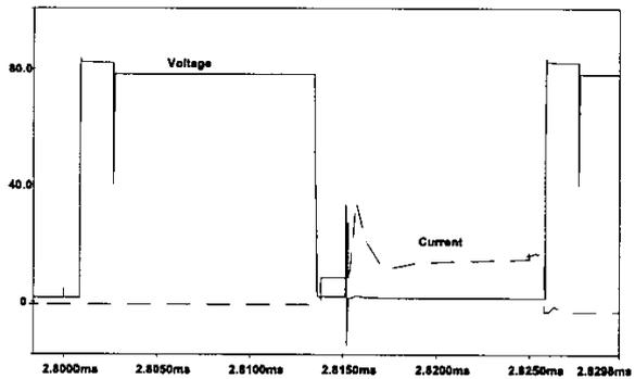
Figure 15 Voltage and current in switch  $S_1$  of the push-pull.
