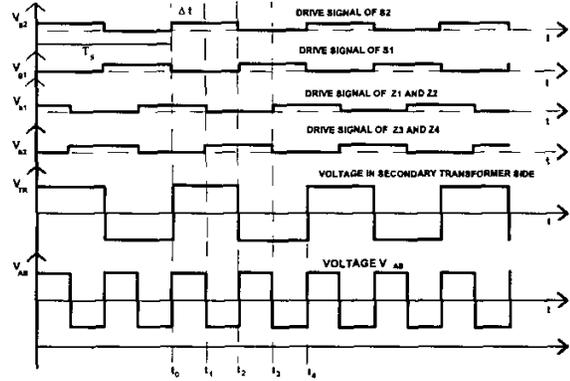
Figure 6 Waveforms for the converter with a fixed phase shift.
