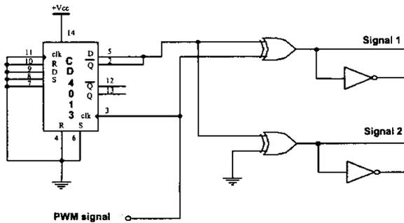
Figure..8 Circuit that generates the time shifting between the two converters
