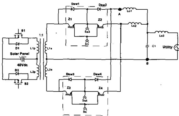
Figure 1. DC/AC converter.
