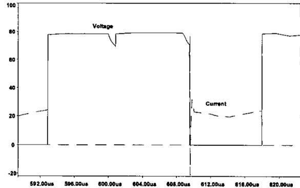
Figure 14 Voltage and current in the first bi-directional set of the cycloconverter.
