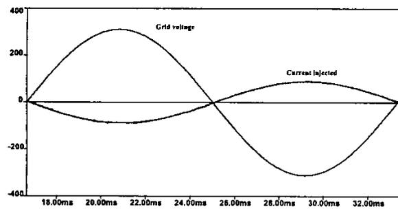
Figure 12 Current and voltage in the main power supply.
