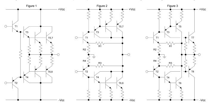
**Figure 1** is a classic triple Darlington stage where each successive transistor is driven from the emitter of the previous stage. This arrangement features a current gain of approximately 10 and a voltage gain of 1. It is reasonable linear but has a few limitations:
