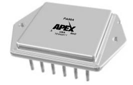
The JEDEC MO-127 12-pin Power Dip<sup>™</sup> package (see Package Outlines) is hermetically sealed and isolated from the internal circuits. The use of compressible thermal washers and/or improper mounting torque will void the product warranty. Please see "General Operating Considerations".
