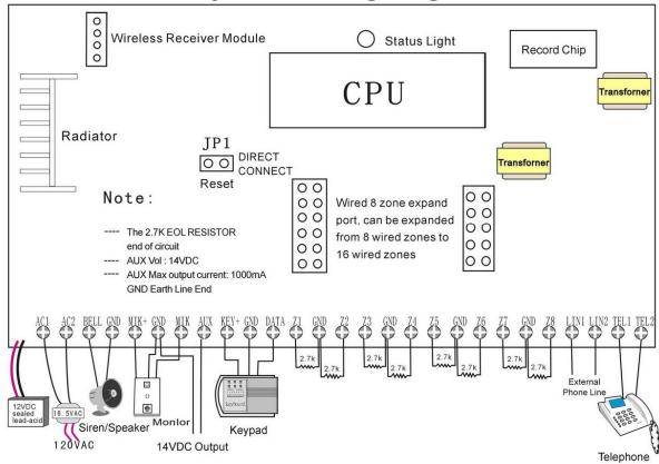
indicator LED will light on when working normally, **Z1-Z8** means 1—8 zone
