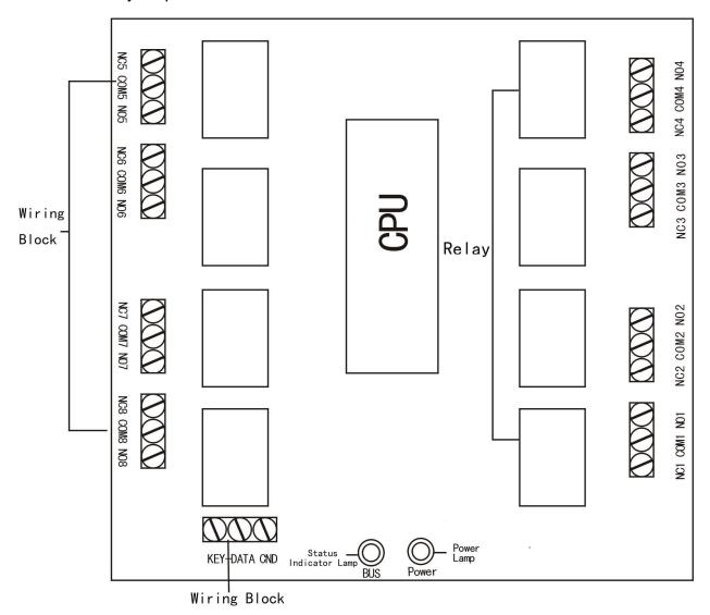
Together 8-way output module with the keyboard connect to the keyboard port, It can customize the output ROADS and OUTPUT methods (Exactly see 4.35) Linkage widely used in monitoring, control of home appliances, and other fields.
