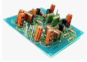
must be equalised following the RIAA standard curve before it is sent to the amplifier. This is necessary because all records today are recorded according to this standard and as the information on the record has the higher frequencies boosted it must be restored to its original shape before we hear it. It is a relatively simple project to build but its performance is Hi-Fi leaving nothing to be desired.
