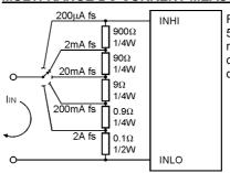
For multi-range, use a 2 pole, 5 way rotary switch. 1 pole for range select and the other to connect the appropriate decimal point to XBP.
