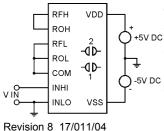
Where a single 5V supply is not suitable but you must connect your O +5V DC input signal ground to the module supply ground, then either of these two non-floating input circuits can be used. -5V DC Note that the module is set in the 9V supply mode.
