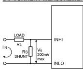
Shunt resistance Rs =  $\frac{Vs}{IIN}$   $\Omega$
