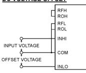
To achieve a zero display reading for a non-zero voltage input, apply the offset voltage between COM and INLO. For a positive offset apply a Positive signal to INLO w.r.t.
