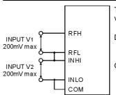
To determine the ratio between two voltages apply the inputs as shown.
