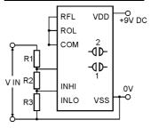
Using the formulae choose resistors to +9V DC ensure the analogue inputs are no closer than 1.5V from either VDD or VSS (VDD-1.5V or VSS+1.5V)
