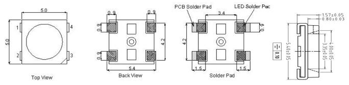
Remarks: Dimension of 5.0\*5.4\*1.57mm, default Tolerance of 0.05mm.
