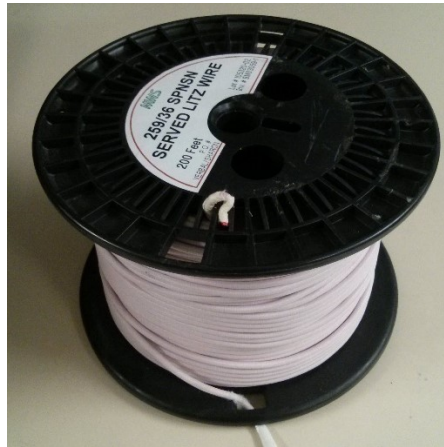
Fig. 4.4. Litz wire 259/36 for transformer prototypes
