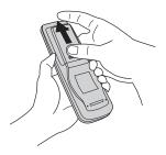
(1) To remove the cover, slide it outwards while pressing it down.
