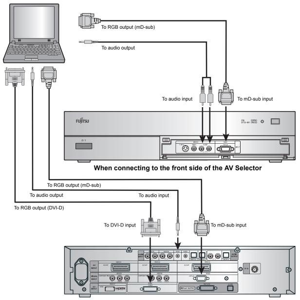
When connecting to the rear side of the AV Selector
