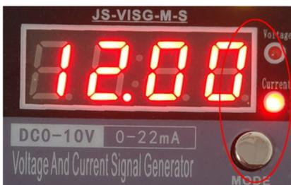
Press The "MODE" Button To Switch Voltage And Current Adjust Mode;
