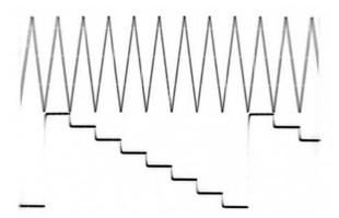
The peak plate voltage is determined by any of the three limit controls. When one of these limits is reached the ramp is reversed back towards OV. Normally the voltage limit control sets the peak voltage. But often you may want to limit either peak current or peak plate power, both of which can occur prior to the voltage limit. This capability is to prevent tube damage.
