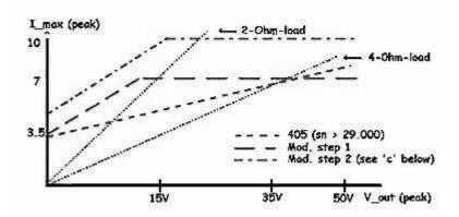
In any case, there probably will not be THD < 0.01% at all 'unprotected' levels after this mod, for sure, and not 50W \_continuous\_ sine-drive into 2 Ohm (so you have to take some care not to overheat the amp when driving low-impedance-loads with continuous signals on the workbench!) -- but there will be no interference by the protection-circuit during for example 7A-peaks into 2 Ohm ( $\sim$ 50W).
