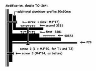
Mount the 3281s (resp. their successors) close to the 40872-side to leave enough room for screw\_1. Place the lower two (T1) first, then add the profile with screw\_1, then the upper two (T2) and at last screw\_2 (the nut on top of T2). All transistor-packages must be insulated with suitable pads and heat-transfer-compound has to be used (even between the profile and the top of T1). To my experience the cooling of all four devices is excellent then.
