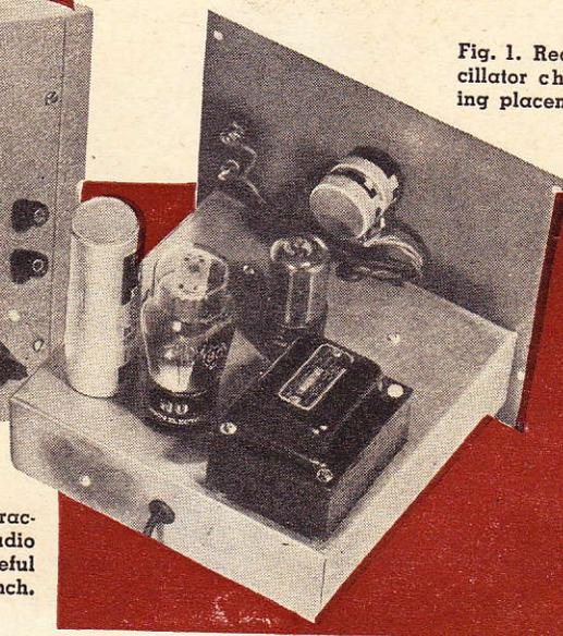
Fig. 1. Rear view of oscillator chassis showing placement of parts.
