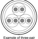
Example of three-pair cable structural drawing
