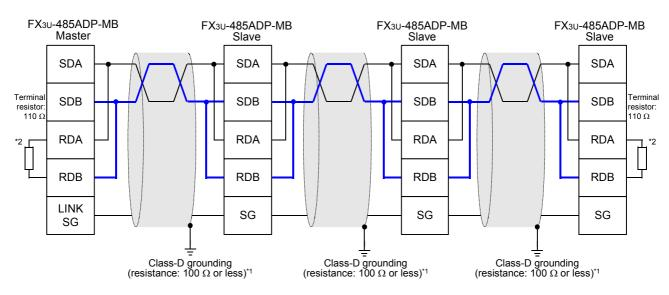
\*1 Make sure to perform Class-D grounding on the shield of the twisted pair cable connected to the FX3U-485ADP-MB.
