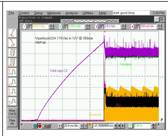
In *Figure 8* the purple trace is the  $V_{dd}$  voltage rising to  $\sim 14$  V. The energy with the  $2.2 \mu\text{F}$  capacitor does not store enough energy. As seen the output voltage (green trace) does not reach high enough to bootstrap. It succeeds the second time after there is a partial charge on the output cap. *Figure 9* is using a  $4.7 \mu\text{F}$   $V_{dd}$  cap. With adequate energy the power supply starts the first time.
