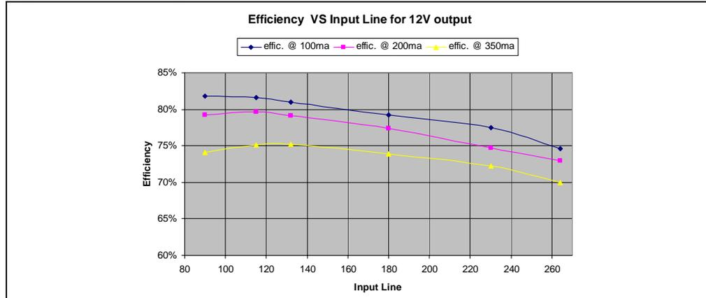
Efficiency is about 75% at 120 V<sub>ac</sub>. Efficiency is better at higher output voltages.
