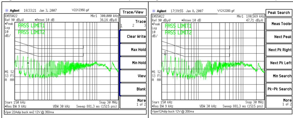
Figure 17. VIPer22-E, 16 V at 350 mA output
