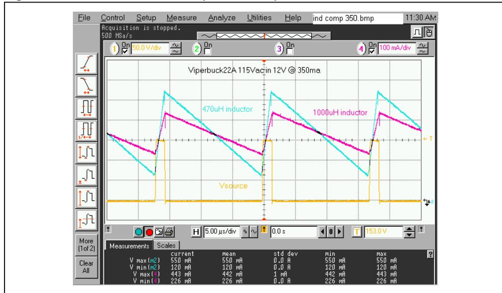
The blue trace is the current with 470  $\mu$ H inductor and the purple trace is the current with a 1000  $\mu$ H inductor.
