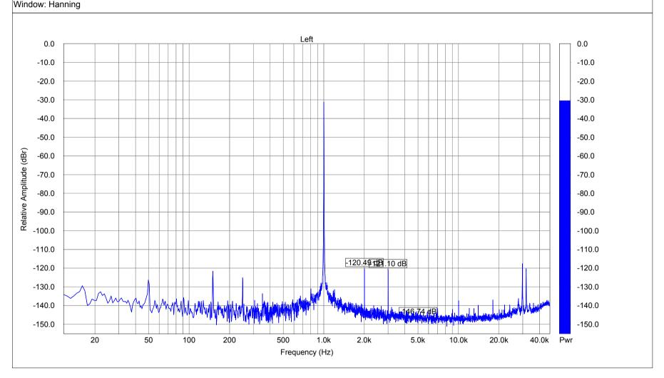
Left Channel Sampling Rate: 96000 FFT size: 131072 Averaging: 10 Window: Hanning TDA7439 5 kHz -20db attenuator Printed By: SpectraPLUS-SC Sound Card Edition Licensed To: msoft Tue Oct 10 23:17:24 2023
