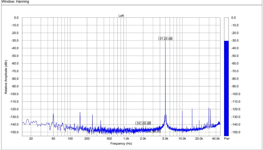
Left Channel Sampling Rate: 96000 FFT size: 131072 Averaging: 10 Window: Hanning TDA7439 10 kHz -20db attenuator Printed By: SpectraPLUS-SC Sound Card Edition Licensed To: msoft Tue Oct 10 23:19:30 2023
